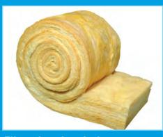
**Fiberglass insulation** comes in batts and rolls or can be blown-in. It can be placed in unfinished walls, floors, and ceilings. It is fitted between studs, joists, and beams.
