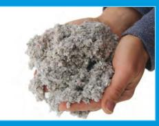
**Cellulose insulation** can be either loose-fill or blown-in. It can be used in existing walls and attic floors.
